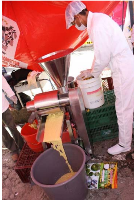
Fruit processing, obtaining chamba pulp. Photo 6. GIDIME Research group.
