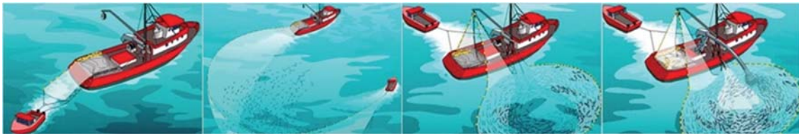
Fig. 1: Phases of Seiner Fishing Operation: Letting, Collecting and Taking the Fish onto the Deck. Source: Denizden Tabaga, June 2014.
