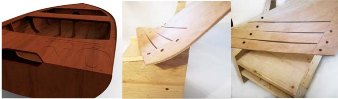
Fig. 1: Render of the first prototyping boat and preliminary tests for the processing of plywood flat panels
