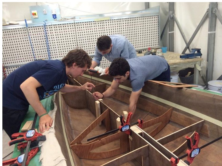
Fig.7: wooden structures in place before their lamination
