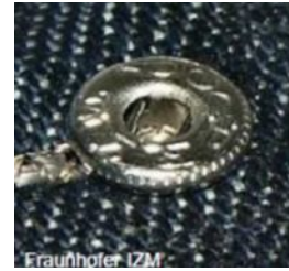
(Fig 5. Unión Force-Fit)[22]
